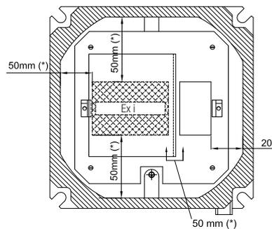
Examples of installation of associated equipment - minimum distances.
